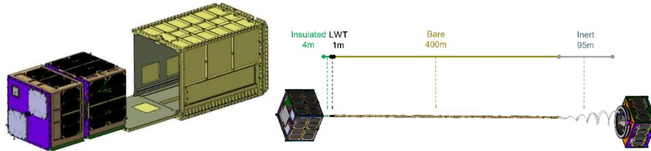
Figure 2. Details of the DK and the longitudinal structure of the tether
