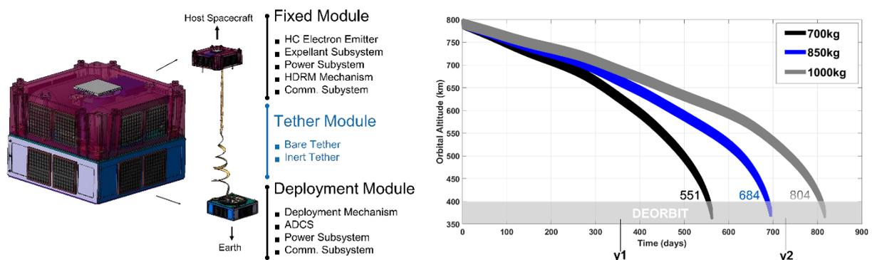
Figure 1. Deorbit kit and its main elements (left) and simulation result of the altitude versus time for a 700-kg spacecraft equipped with a 35-kg deorbit kit.
